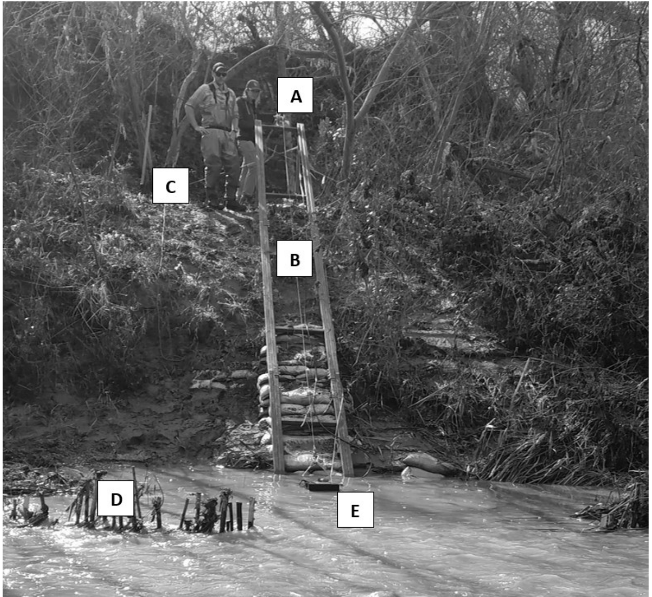
Figure 2 Salsipuedes Creek DIDSON deployment track system in 2017 with key features labeled. (A) winch; (B) track; (C) cross-bracing cables; (D) deflection panels; (E) DIDSON/X2/sled assembly.
